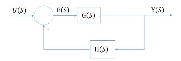
Plot the root loci for the closed-loop control system?
