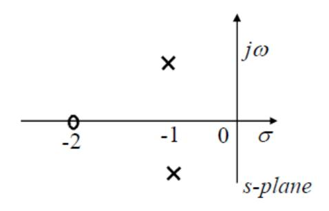
2. Determine the root loci on the real axis: Root loci exist on the real axis between -2 and  $-\infty$ .
